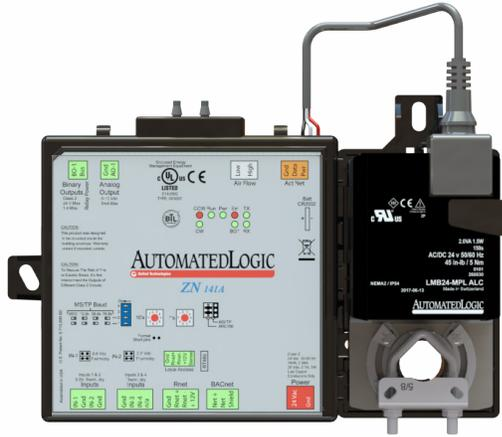
The ZN141A is a fully programmable, native BACnet Advanced Application Controller that provides zone level temperature and air quality control for pressure-independent VAV applications. Sophisticated pre-engineered control algorithms reduce energy consumption, extend actuator life, and increase occupant comfort. It communicates on an EIA-485 LAN using BACnet MS/TP or BACnet over ARCNET communications and connects seamlessly to the WebCTRL® building automation system.
