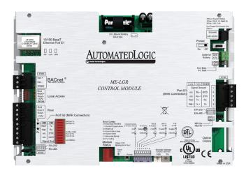
The Automated Logic ME-LGR controllers are an integral component of the WebCTRL® building automation system.
