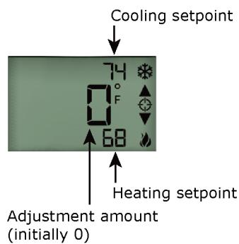
**NOTE** The control program may not show the cooling and heating setpoint on this screen.
