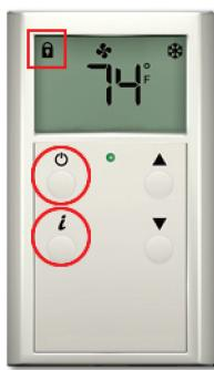
Press and hold the 2 buttons again for 5 seconds to unlock the buttons.
